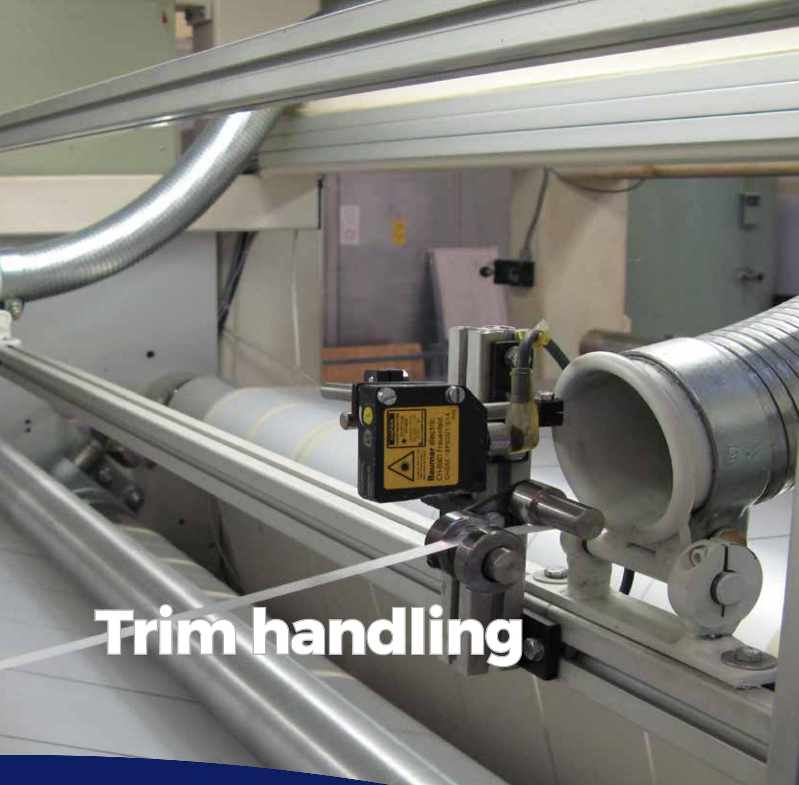
A close-up photograph of industrial machinery. A white cylindrical component is connected to a metal pipe. A black and yellow Baumer electric sensor is mounted on the machinery. A thin white strip of material is being processed. The background shows a factory setting with metal frames and pipes.
